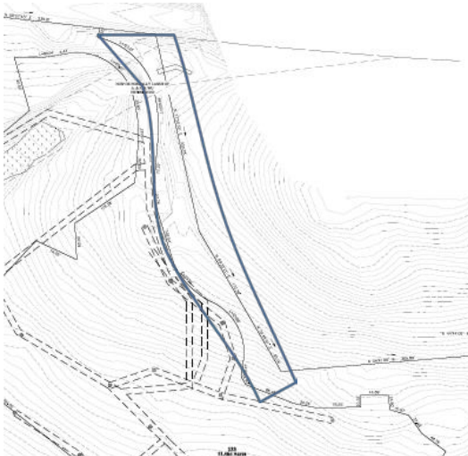
Figure 3: Detail of PL-1.05, with a long narrow strip applicant proposes to be created by subdivision. This strip ranges from 23 to 60 feet in width and is about 600 feet long
